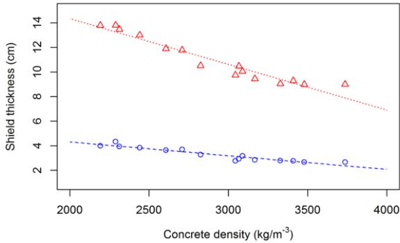
Fig. 1. Variation of HVL and TVL values, gamma attenuation estimators, as a function of the density of different concretes for a  $^{137}\text{Cs}$  source.
