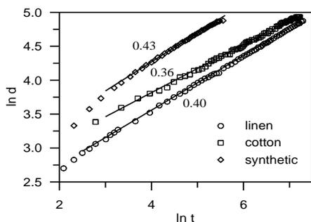
Fig. 1. Logarithmic plot of the wetting front distance from the water immersed end of a cotton fabric as a function of time. The numbers are the values of the  $\alpha$  exponent.
