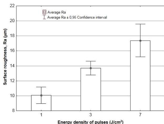
Fig. 3. Influence of the energy density of pulses on surface roughness.
