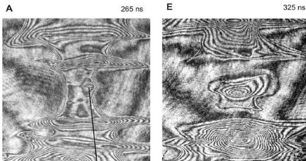
Fig. 5. Interferometric images of different phases of shot #11189: (A) - constriction of plasma column, (E) - the pinch interruption and formation of separate plasmoids.
