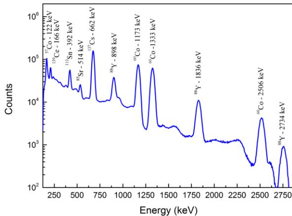
Fig. 1. Calibration spectrum recorded with a  $3'' \times 3''$  CeBr<sub>3</sub> scintillator at JET.
