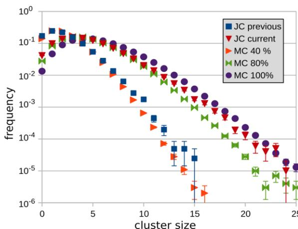
Fig. 2. Ionization cluster-size distributions for 3.8 MeV alpha particles irradiating a 0.32 µg/cm<sup>2</sup> nitrogen target.
