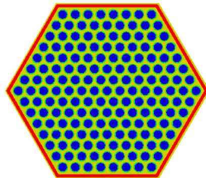
Fig. 1. ALLEGRO fuel assembly model in the SCALE6.2/TRITON.
