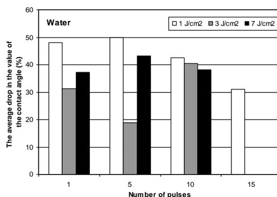
Fig. 1. The average drop in value of the contact angle vs. number of pulses and pulse energy density.
