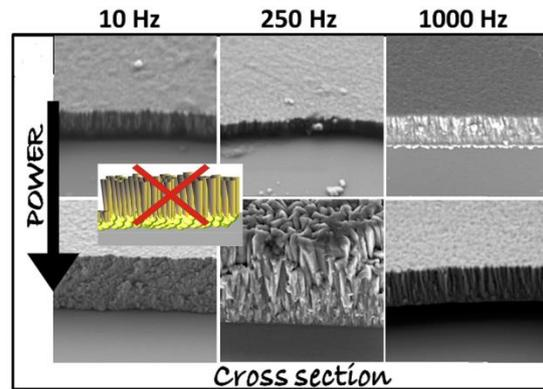
Fig. 2. Cross section views of the Cu-N layers.
