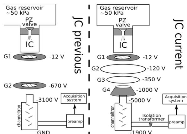
Fig. 1. Schematic layouts of the previous (left) and current setups of the Jet Counter with the key changes (not to scale).
