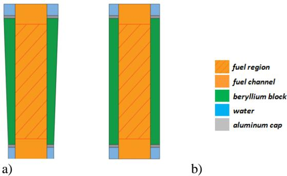
Fig. 1. Schematic vertical section of MARIA beryllium block with fuel element. (a - realistic, b - simplified).
