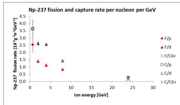
Fig. 2. Np-237 fission and capture rate per ion's nucleon for various ion beams. The symbols in the legend stand for fission (F) or capture (C) per beam ion (p, d, C6+)
