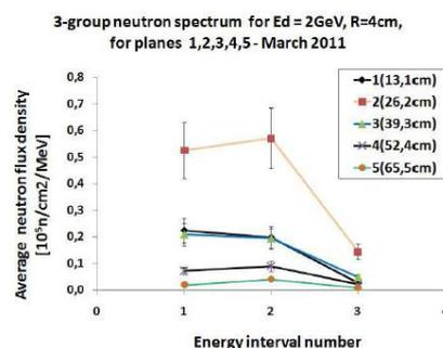
Fig. 3. Average neutron flux density versus three different energy ranges: 1- (11,5-20,8 MeV), 2- (20,8-32 MeV), 3- (32-100MeV) for  $R=4$  cm and five planes (number of successive planes 1,2, 3, 4 and 5); deuteron beam energy 2 GeV;
