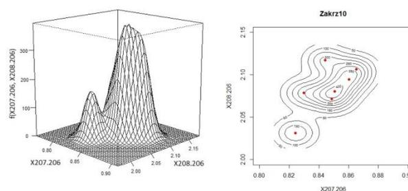
Fig. 2. 3D and 2D lead isotope ratio. Distribution for one object after statistical treatment. Dispersion of results indicates that secondary smelting may have been used.
