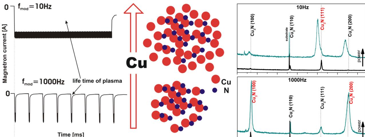
Fig. 3. Schematic illustration of the influence of the duration of each plasma pulse, on the sputtering phase duration (left). The X-ray diffraction patterns of the Cu-N layers- phase composition.
