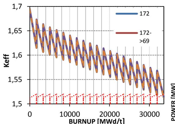
Fig. 2. Effective multiplication factor as a function of burnup. The effective multiplication factor comparison for the APOLLO2 calculations is presented in Fig. 2. Reactor cycles are presented with power changes.
