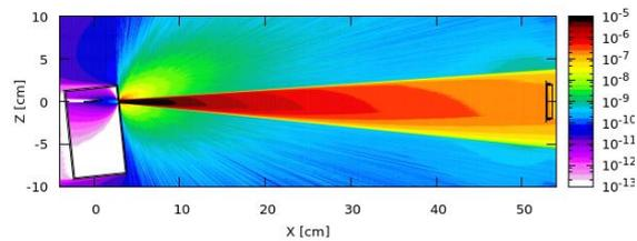
Fig. 3. Dose equivalent in pSv/Ne0 in the second stage of the calculation. The size of the test Petri dish is smaller than the dimensions of the main photon beam.
