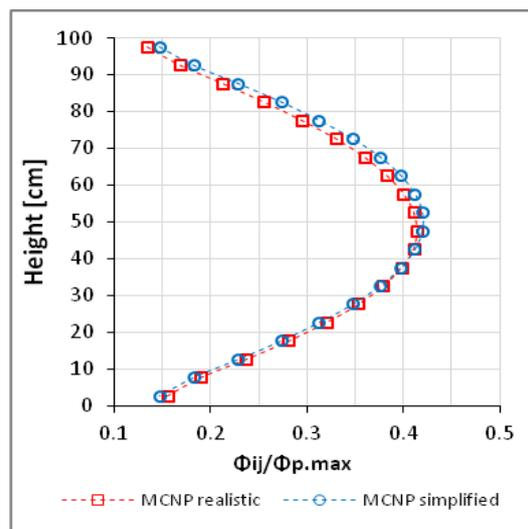
Fig. 4. Comparison of MCNP fast fluxes in fuel for realistic and simplified models.
