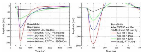
Fig. 1. Example of the output pulses recorded using an oscilloscope, at 50 ohms, for a detector consisting of a 10x10x5 mm<sup>3</sup> LSO read by 4x4 (red), 8x4 (blue), 8x8 (green) and 16x16 (black) channels selected in the 16x16 channel MPPC array.
