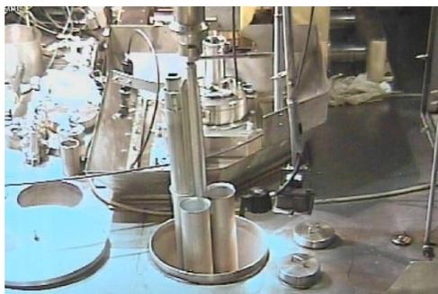
*Fig. 1. Operation of transferring the MR type SFA from the storage pool into the disassembly cell.*
