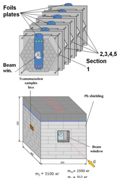
Fig. 1. Schematic of the Quinta assembly. Above view of the uranium target with supporting structures and plastics used for sample placement (detector plates). Below: view of the lead shielding encasing the target with the location in the shielding of the transmutation samples box (window) for the actinide sample marked.
