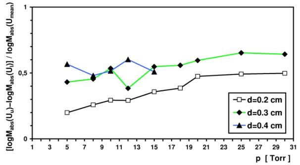
Fig. 4. Relative variability dynamics of effective gas amplification within the PPAC ER-plateau range; the  $U_{\text{mean}}=(U_l+U_w)/2$ -supply voltage relates to the detector ER-plateau range (see fig. 3).
