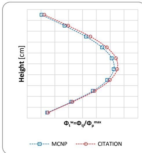
Fig. 6. Neutron flux distributions for MCNP and improved CITATION models thermal flux.
