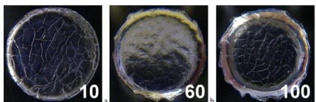
Fig. 4. Pictures of the front surface of a single rod from the centre of the W-brush target after its irradiation by 10, 60, and 100 plasma pulses in the QSPA facility.
