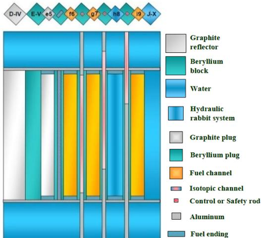
Fig. 2. Schematic vertical section of the MARIA core.
