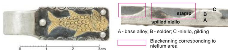
Fig. 1. Belt hanger with fish representation: view of the surface (left) and MO cross section of artifacts (right).
