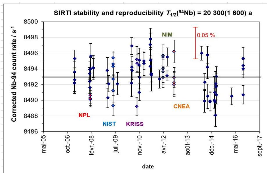
Fig. 3. Results of  $^{94}\text{Nb}$  control source measurements in SIRT. The most recent points on the graph represent measurements made at RC POLATOM.
