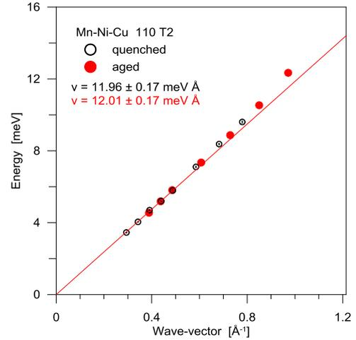
Fig. 2. The low energy part of the transverse T2 phonon dispersion relation in the [110] direction for a homogenised sample and after short ageing.
