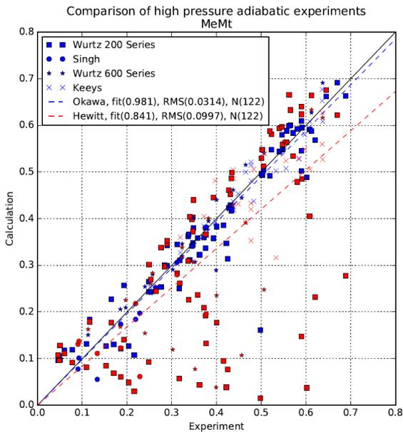
Fig. 1 Comparison of experimental and simulated data for adiabatic experiments.
