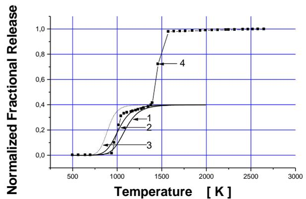
Fig. 2. Temperature dependences of helium release from the  $UO_2$  surface. The solid curves of the quantum variant are: 1: based on the “ab initio” calculation; 2: corrected, according to the best fit to the experimental data; 3: the dashed curve 3 is the classic variant. 4: experimental data from [2].
