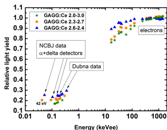
Fig. 1. Non-proportionality of the GAGG:Ce scintillators measured over a wide energy range.
