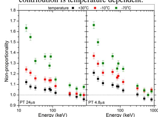
Fig. 1. Non-proportionality characteristics of a tested CsI:Tl crystal measured at two peaking times in the amplifier. Data presented for CsI:Tl scintillator with Tl concentration equal 0.032% mole, at three temperatures:  $+30^\circ\text{C}$ ,  $-10^\circ\text{C}$  and  $-70^\circ\text{C}$ .
