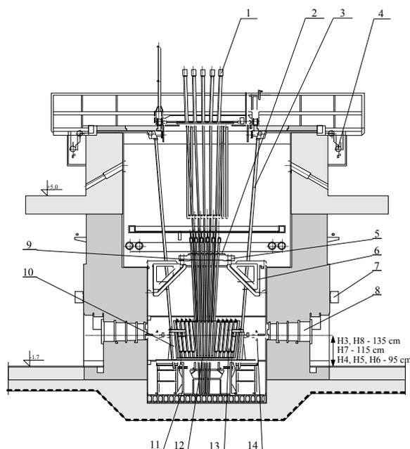
Fig. 1. Vertical section of the MARIA reactor. 1. control drive mechanism, 2. mounting plate, 3. ionization chamber channel, 4. ionization chamber drive mechanism, 5. fuel and loop channels support plate, 6. plate support console, 7. horizontal beam tube shutter drive mechanism, 8. beam tube shutter, 9. fuel channel, 10. ionization chamber shield, 11. core support structure, 12. core and reflector support plate, 13. reflector blocks, 14. beam tube compensation joint.
