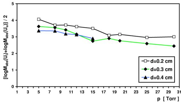
Fig.3. Mean effective gas amplification change within the PPAC ER-plateau range; for the  $U_l$  and  $U_w$ -supply voltages see text.
