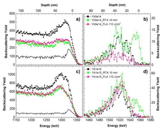
Fig. 1. Random and aligned RBS/c spectra for a ZnO single crystal implanted with Yb ions to fluencies of  $5 \times 10^{14}$  (a,b) and  $1 \times 10^{15} / \text{cm}^2$  (c,d) in the as-implanted stage and after different types of annealing. RTA were performed at  $800^\circ \text{C}$  for 10 min and FLA for 20 ms with flash energy of  $110 \text{ J/cm}^2$ .
