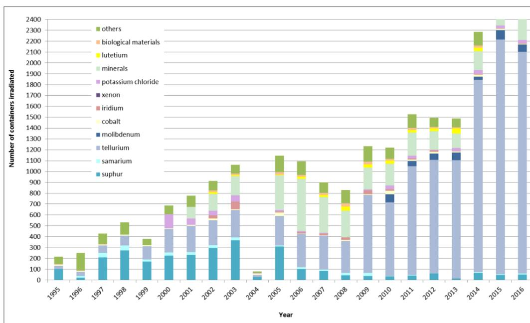
Fig. 7. Distribution of irradiated target materials.
