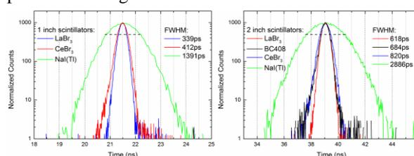
Fig. 2. Normalized timing spectra recorded with a detector consisting of 1 inch (left) and 2 inch (right) scintillators: LaBr<sub>3</sub> (red), CeBr<sub>3</sub> (blue) and NaI(Tl) (green) read by 16x16 channels of the MPPC array.
