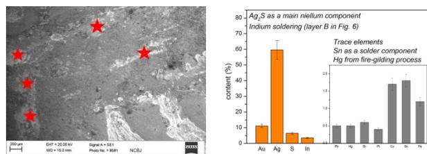
Fig. 2. (left) SEM image with corrosion cavity (in the range of  $\mu\text{m}$ ) which allows layer composition to be determined: A, B, C on Fig. 1 and the presence of higher indium content in cavities: B and average results of SEM/EDX  $\mu$ -analysis of belt hanger (right).
