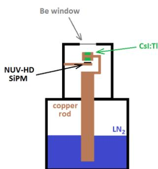
Fig. 1. The LN<sub>2</sub> cryostat with the CsI:Tl crystal and the NUV-HD SiPM mounted on separate copper frames.
