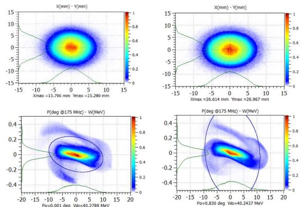
Fig. 1. Comparison of beam distribution. Top: X-Y space; bottom: phase-energy space; left: GPT results; right: TraceWin results.
