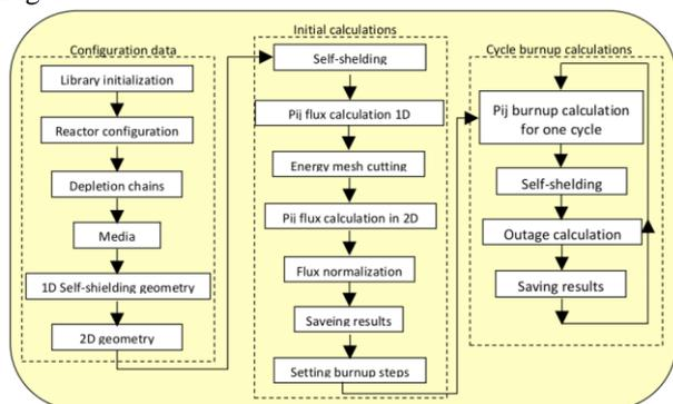
Fig. 1. Data flow for the Collision probabilities method in the APOLLO2 code.
