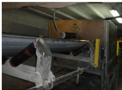
Fig. 2. The test installation of the RaM-scaN system demonstrator on a conveyor belt in the "Folwark" mine in Poland.
