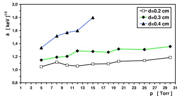
Fig. 1 Mean values of the constant  $k$  – relating to individual plateau ranges of PPAC energy resolution – vs. n-heptane pressure. The change in pressure was accompanied by a simultaneous change in the specific ionization (see ref. [3]).
