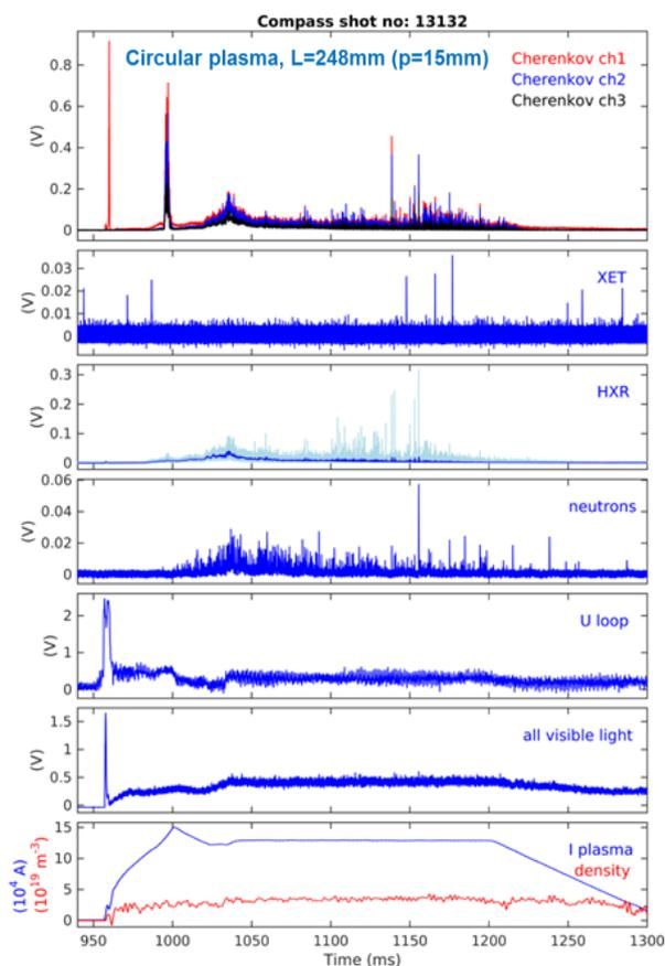
Fig. 1. Comparison of hard X ray signals (HXR), photo-neutrons,  $U_{loop}$  and visible light emission with electron-induced signals from a three-channel Cherenkov probe (intensity [V] versus time [ms]). The plasma current was positive, and density reached  $3 \times 10^{19} \text{ m}^{-3}$ .
