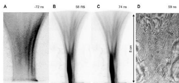
Fig. 4. XUV images recorded at various instants of shot #11200: (A) at -72 ns, (B) at +58 ns, (C) at +74 ns. The interferometric image (D) was taken at the same instant as (B), and its upper part also showed some filaments.
