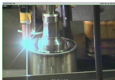
*Fig. 3. Operation of the first weld in the disassembly cell.*
