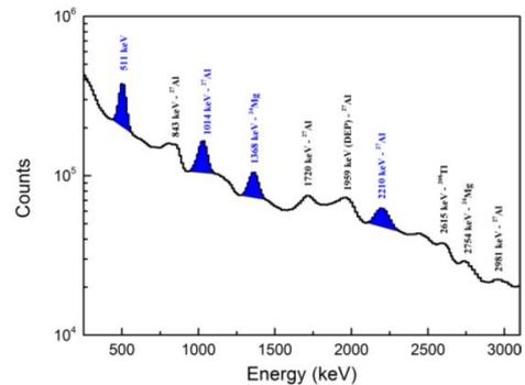
Fig. 2. Typical spectrum obtained at LNL for a  $20 \times 15 \text{ mm}^2$   $\text{CeBr}_3$  coupled to an MPPC, with a TIA and MTCD measured at 30 nA current with a maximum rate of  $\sim 340 \text{ kHz}$  for 120 s.
