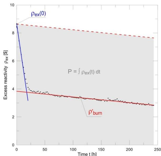
Fig. 1. Initial excess of reactivity and rate of decrease in reactivity, for one of the operating cycles of the MARIA reactor. The real excess of reactivity has been highlighted in grey.
