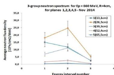
Fig. 2. Average neutron flux density versus three different energy ranges: 1-> (11,5-20,8 MeV), 2-> (20,8-32 MeV), 3-> (32-100MeV) for  $R=4$  cm and five planes (number of successive planes 1,2, 3, 4 and 5); proton beam energy 0.66 GeV.
