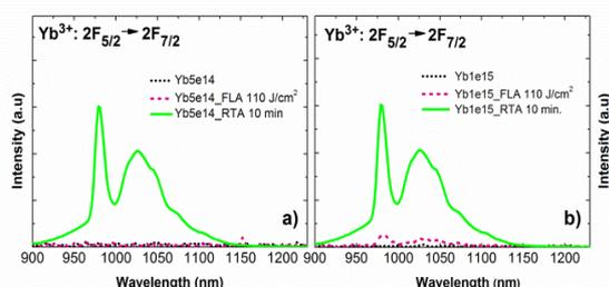
Fig. 2. RT PL spectra for a ZnO single crystal implanted with Yb ions to fluencies of  $5 \times 10^{14}$  (a,b) and  $1 \times 10^{15} / \text{cm}^2$  (c,d) for as-implanted sample and after different types of annealing. RTA was performed at  $800^\circ\text{C}$  for 10 min and FLA for 20 ms with flash energy of  $110 \text{ J/cm}^2$ .
