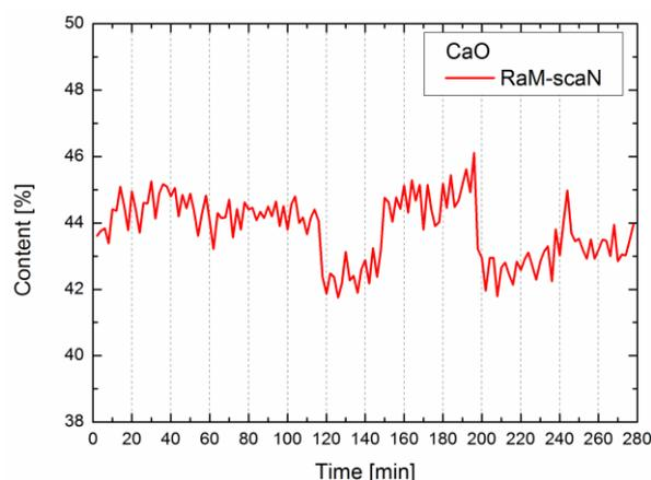
Fig. 3. Preliminary results of calcium oxide content calculations on the basis of the RaM-scaN demonstrator data.
