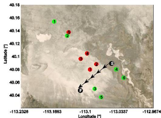
Fig. 1. Topographic map of the OLAD Trial-252-2 experiment. The black dots mark the starting (S) and final (F) points of the release; The sampling points are indicated with red dots and the weather stations with green squares. (39.9800N, 113.2 W).
