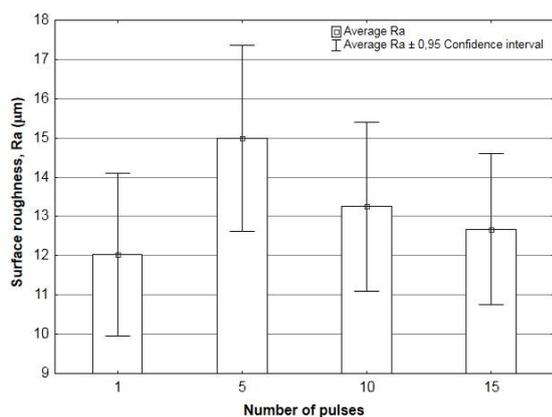
Fig. 2. Influence of the number of pulses on surface roughness.
