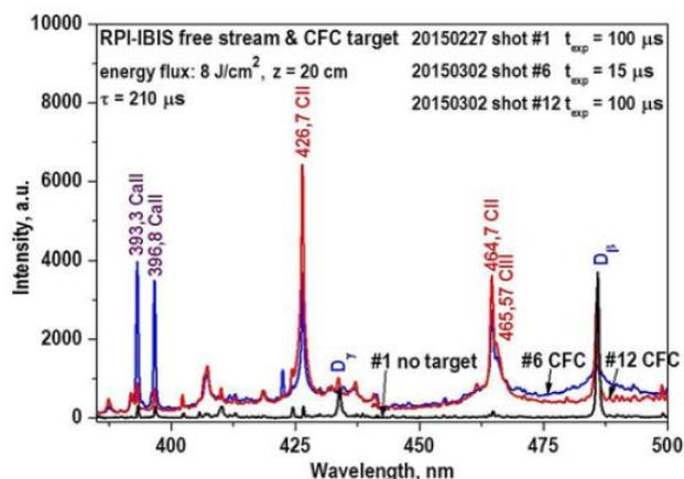
Fig. 2. Comparison of optical spectra from a free plasma stream (black) and those from 2 shots performed with the CFC target (blue at  $t_{exp} = 15$   $\mu$ s, red at  $t_{exp} = 100$   $\mu$ s).
