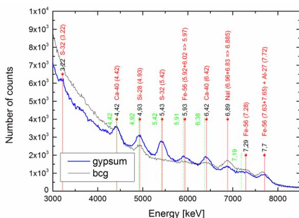
Fig. 1. Example of the PGNAA spectrum of a gypsum sample (from a cement plant in Kazakhstan) registered at NCBJ using a laboratory setup.
