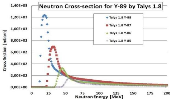
Fig. 1 Microscopic cross sections calculated by the TALYS 1.8 code for the  $^{89}\text{Y}(n, xn)$  reactions.
