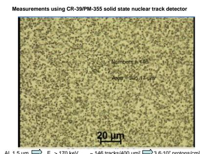
Fig. 2. Tracks induced by energetic protons in a sample of PM-355 nuclear track detector.
