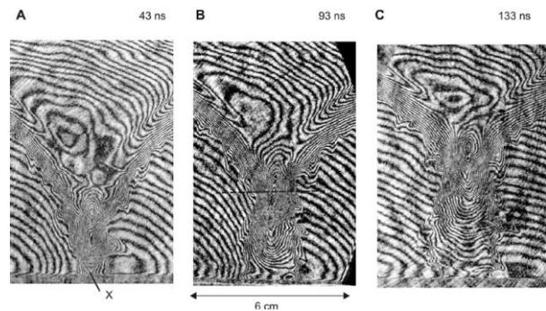
Fig. 7. Interferometric images of shot #10912 with He-filling, as recorded: (A) at the SXR maximum, (B) after HXR peak maximum, (C) after all the X-ray pulses.
