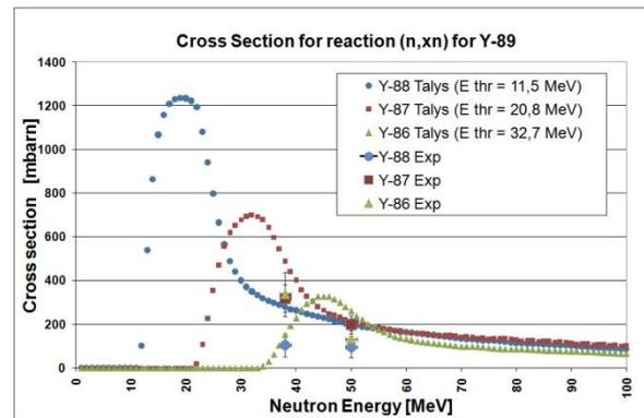
Fig. 2 Comparison of  $^{89}\text{Y}$  (n,xn) cross-section measurements and calculations. Our Uppsala experiments in 2015 are represented by the six bigger points. TALYS 1.8 [4] calculation results are represented by circles ( $^{88}\text{Y}$ ), squares ( $^{87}\text{Y}$ ) and triangles ( $^{86}\text{Y}$ ).
