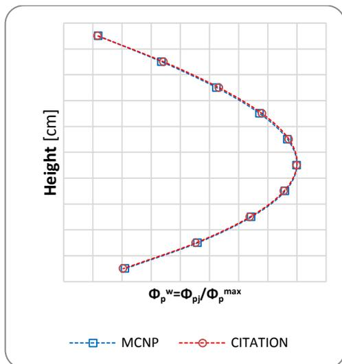
Fig. 5. Neutron flux distributions for MCNP and improved CITATION models, fast flux.
