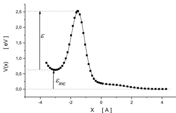
Fig. 1. The potential of the crystalline field,  $V(x)$  of He atoms versus distance from the surface,  $x$ .
