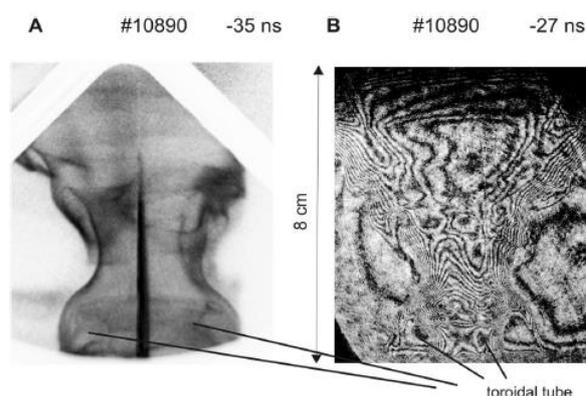
Fig. 3. Toroidal micro-structures inside the Al-wire corona and dense plasma column during the first SXR-pulse emission, as observed: (A) on the XUV frame, (B) on the interferometric image.
