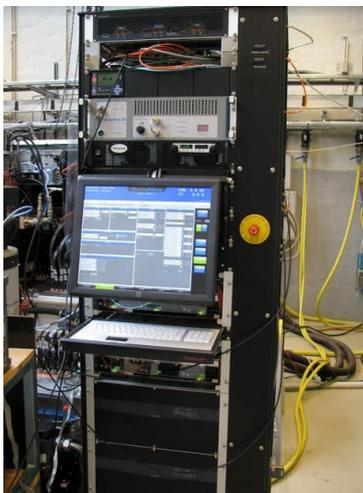
Fig. 2. Klystron modulator during FAT.
