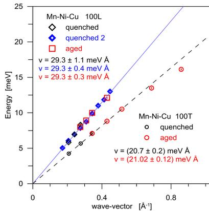
Fig. 1. The low energy part of the longitudinal and transverse phonon dispersion relation in the [100] direction investigated in a homogenised sample and after short ageing.
