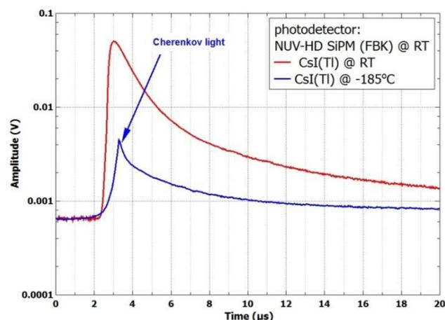
Fig. 2. CsI:Tl scintillation decay profiles measured at RT (red line) and at -185°C (blue line).
