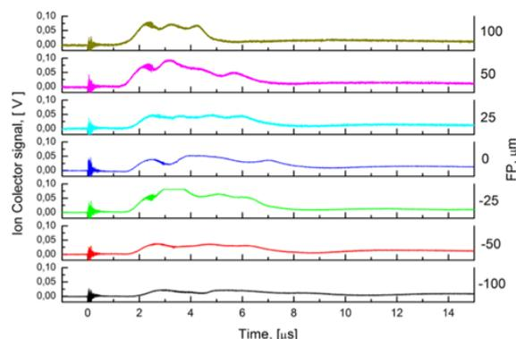
Fig. 3. Mylar foil target. Ion collector signals in dependence of the laser focal position with respect to the target surface.
