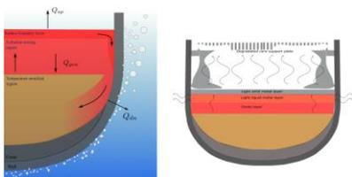
Fig. 1. Heat transfer during the IVMR strategy. Focusing effect.
