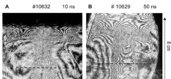
Fig. 2. Interferometric images recorded during the stagnation of the pinch column: (A) for shot #10632 performed with the Al-wire, (B) for shot #10629 without any wire.
