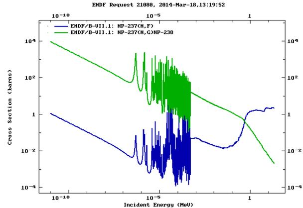
Fig. 1. Np-237 neutron induced fission (dark blue) and capture (green) cross section dependence on energy.
