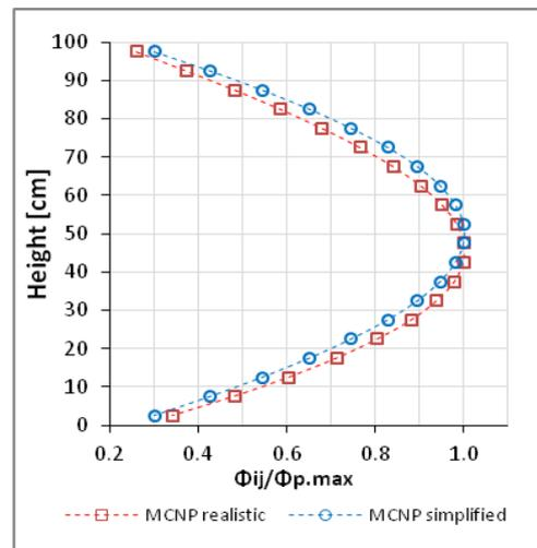
Fig. 3. Comparison of MCNP fast fluxes in fuel for realistic and simplified models.
