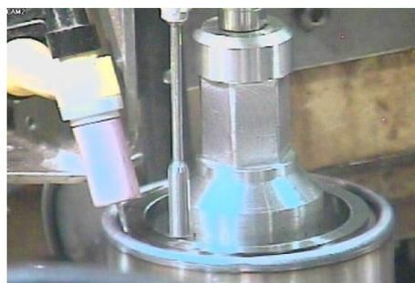
*Fig. 4. Operation of checking the tightness of the first weld.*
