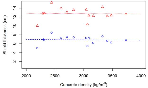
Fig. 2. Measured values of 1.HVLn (circles) and 1.HVLn+2.HVLn (triangles) for various types of high performance concretes. Measured results do not show any correlation to concrete density.
