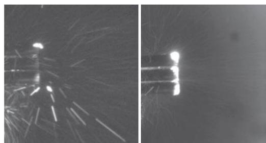
Fig. 3. High-speed pictures of the tungsten brush-like target, which were taken during the 20<sup>th</sup> shot (left) and during the 30<sup>th</sup> shot (right), at  $t = 3.6$  ms after the irradiation start, and at a frame exposure time equal to 1.2 ms.
