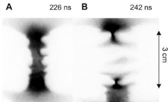
Fig. 6. Shot #11200. XUV images from shot #11200, which show the final phase of a regular constriction: (A) - before the HXR and neutron emission, (B) - during this emission.
