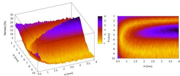
Fig. 2. The function  $f(H,R)$  calculated in a model of the complete beam forming system depicted in Fig. 1.
