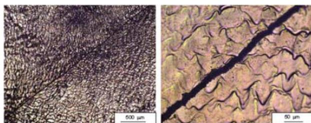
Fig. 1. Pictures of the W-sample surface (at different magnifications) which was placed at a distance of 6 cm from the PF-1000U electrode outlets and irradiated by 3 plasma shots performed at  $p_0 = 1,6$  hPa ( $D_2$ ) and  $U_0 = 21$  kV.
