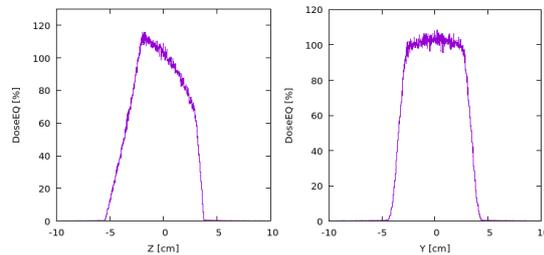
Fig. 4. Sections of the photon beam obtained in the segment detector plane along the Y and Z axes.
