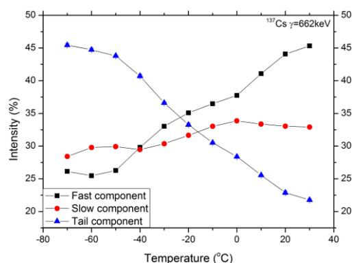
Fig. 2. Intensities of three light pulse components. Data presented for CsI:Tl ( $x_{Tl} = 0.032\text{mole}\%$ ) with  $^{137}\text{Cs}$   $\gamma$  source (662keV).
