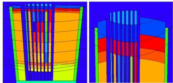
Fig. 2. Vertical cross-section of the MCNP core model, vertically contracted for demonstrating the layers. Convex – fuel element layers, concave – graphite matrix layers. Left – whole core height, right – focus on the top part.
