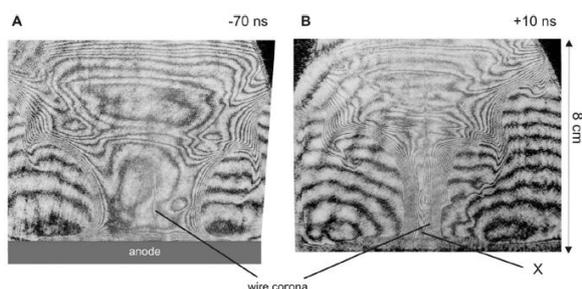
Fig. 1. Interferometric images from shot #10633, obtained: (A) at the current sheath implosion, (B) at the formation of the 1st dense plasmoid.
