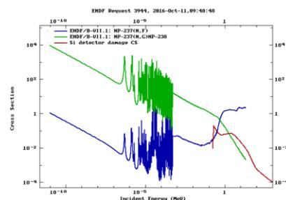
Fig. 2. Cross section of neutron inducing damage in the silicon detector (red curve) and cross sections of neutron induced fission and capture on the Np-237 minor actinide.
