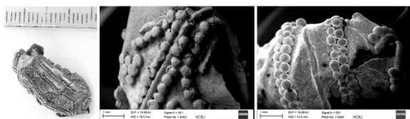
Fig. 1. Photo of jewelry: granulated silver bed, SEM images of surface with granulate mounting to surface by copper-tin solder. EDX results (wt%) Ag/Cu/Sn: 74.7/3.0/0 for surface, 73.9/2.1/0.7 for granulate and for solder 1.7/23.4/7.4 with higher content of oxygen 38.1 (hot treatment).
