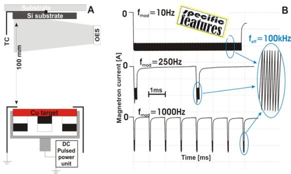
Fig. 1. Schematic view of the experimental setup and current waveforms that show the pulsed manner of plasma generation by the PMS method.
