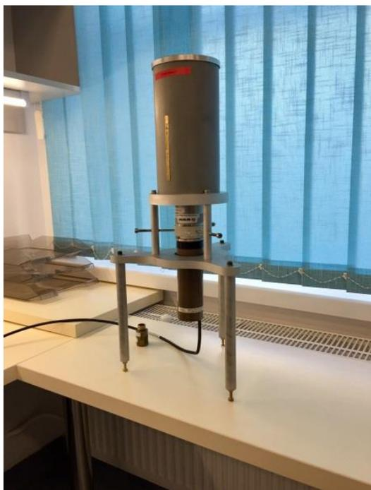
Fig. 2. SIRTI instrument used during the international comparison of short-lived radionuclide activity measurements.
