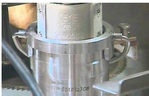
*Fig. 2. Identifying the number on the capsule and the number of the SFA.*
