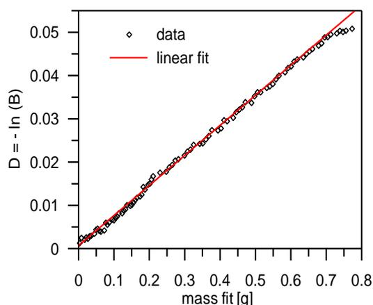
Fig. 2. The dependence of the average optical density in the image and the mass of the sample for the drying of linen.
