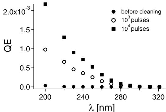
Fig. 2. Quantum efficiency results for an arc coated and pulsed plasma annealed photocathode.
