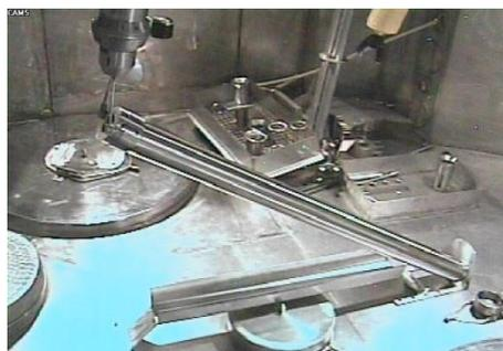
*Fig. 5. Operation of reversing the capsule on the cradle.*
