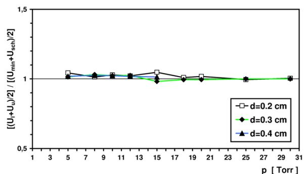
Fig. 2. Ratios of the PPAC detector supply voltage mean value change within the detector ER-plateau range to the PPAC voltage mean value change within the effective gas amplification linear variability range in a semilogarithmic coordinate system; for the  $U_b$ ,  $U_u$ ,  $U_{min}$  and  $U_{sch}$ -supply voltages see text.
