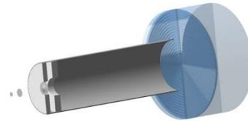
Fig. 1. Geometry model. From left to right: accelerator exit window, scattering foil, flattening foil (Gaussian shape), steel flange, tubular applicator and a water phantom for dose calculation. (See [4] for details).
