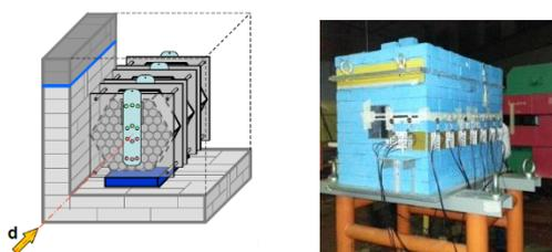
Fig. 1. The QUINTA assembly (left) a cut-away view of the uranium target with supporting structures and plastics used for sample placement; (right) view of the lead shielding enclosing the target.
