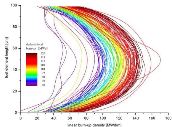
Fig. 1. Measured space distribution of burn-up of spent fuel assemblies; the warmer the colour, the higher the declared burn-up.
