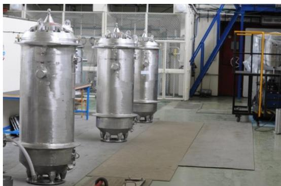
*Fig. 1. TUK-19 containers in the MARIA reactor decontamination hall.*
