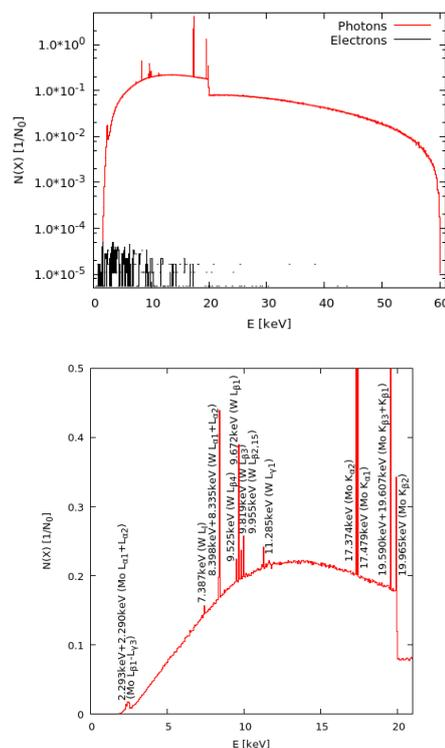
Fig. 2. Photon beam spectrum on the Be window. One can see the characteristic radiation emitted from Mo and the L series from W.
