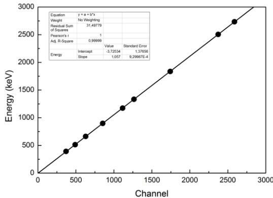
Fig. 2. Energy calibration of the spectrometer based on the CeBr<sub>3</sub> scintillator. Solid line is a linear fit to the experimental points.
