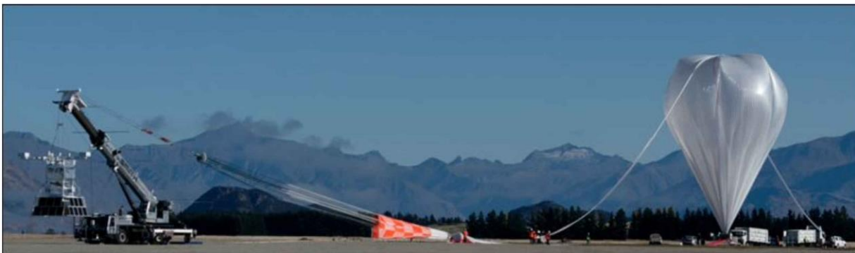
Fig. 1. EUSO-SPB detector during preparation (Wanaka - New Zealand). Detector mounted in gondola of stratospheric balloon provided by NASA observed Earth's atmosphere during 12-days flight for searching of cosmic rays signals [5].
